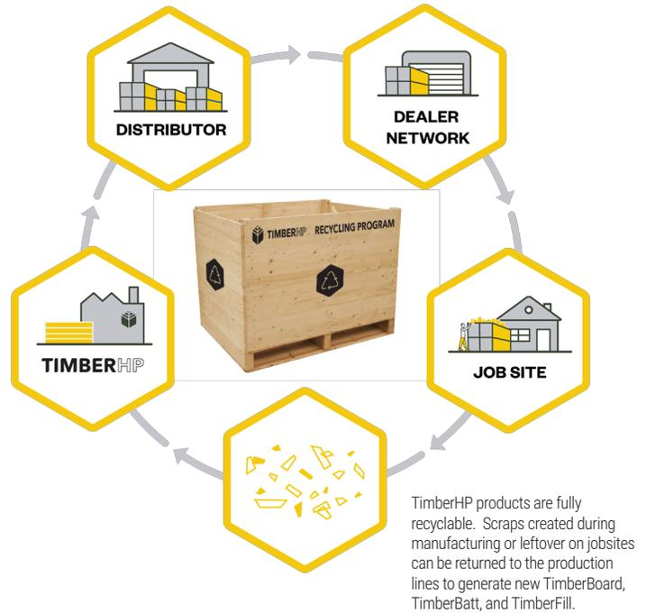
they will be cleaned, refined, and turned into wood fiber insulation. These recycled scraps are considered certified sustainable under the FSC Chain of Custody rules.
