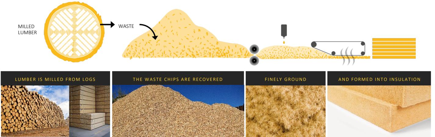
Our manufacturing facility converts wood waste from sawmills and chips from low-value, small-diameter trees into high-value insulating composites
