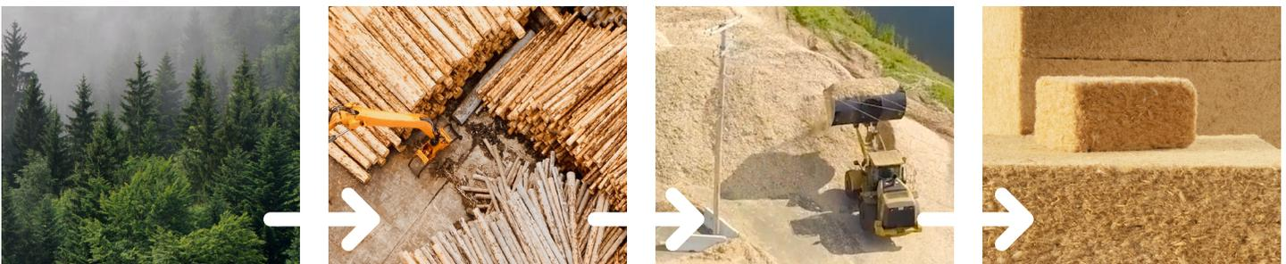
TimberHP wood fiber insulation is produced from the waste stream of the forest products industry.
